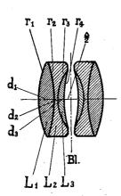
$$\begin{bmatrix} L^{1}_{\gamma 2}^{-1} = +19.5 & d^{1} = 3.4 & nD = 1.6584 & nG = 1.6825 \\ L^{2}_{\gamma 2}^{-1} = \pm 28.2 & d^{2} = 0.8 & nD = 1.5991 & nG = 1.6196 \\ L^{3}_{\gamma 4}^{-1} = -23 & d^{3} = 1.4 & nD = 1.4634 & nG = 1.4723 \\ & \frac{\Delta}{2} = 1.6 \\ Image angle about 100°. Aperture ratio 1:9 \\ Focal length 100°.$$
